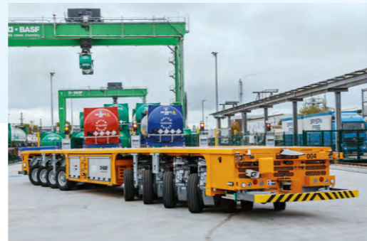
BASF SE: Automated guided vehicles (AGV)
