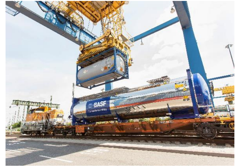
Standard tank container 25,000-36,000 liter volume 25 tons payload
