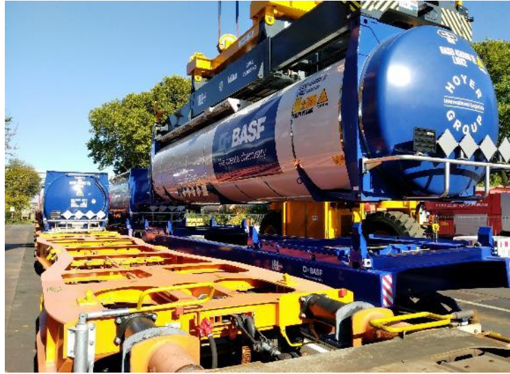
BASF Class Tank Container up to 73,000 liter volume 66 tons payload
